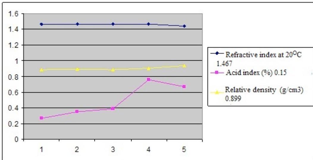
Figure 1. Variation of the refractive and acid indices of the palm oil treated in the microwave
