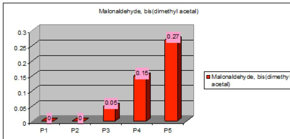
Figure 4. Concentration of malonaldehyde from the palm oil samples treated in a microwave
