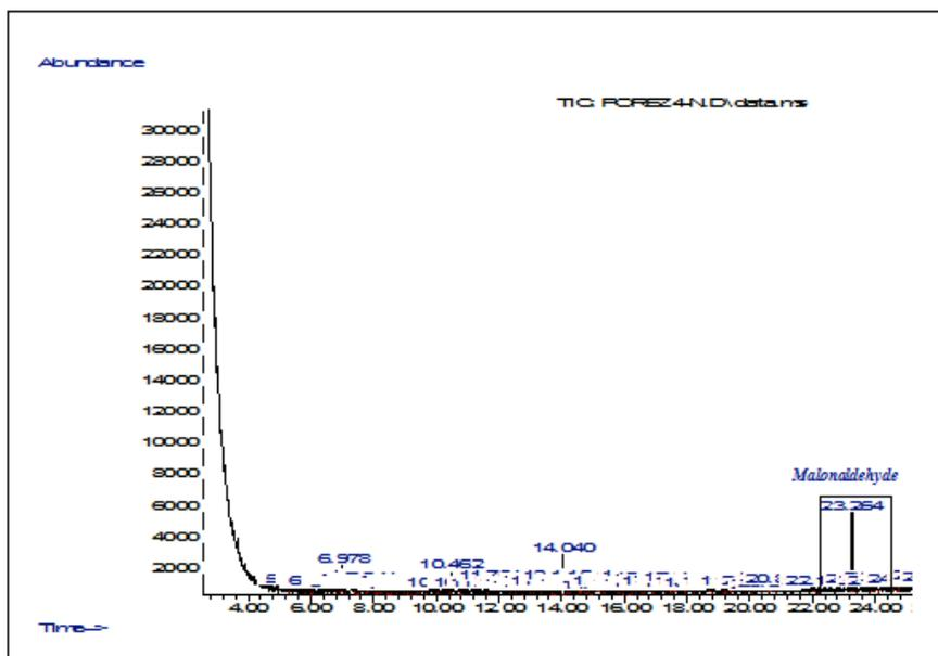
Figure 3. Gas chromatography from the GC-MS analysis of the palm oil treated for 20 minutes in the microwave
