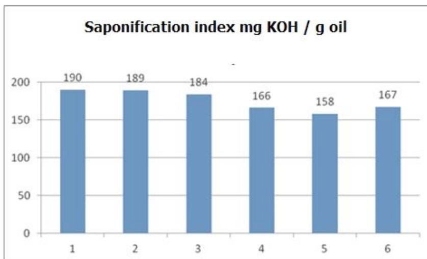
Figure 2. Saponification index variation in the palm oil treated in the microwave
